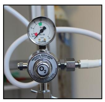
The O2 hose pipe connected to the oxygen manifold on the RM3 can be connected to the regulator on the bottle and tightened
